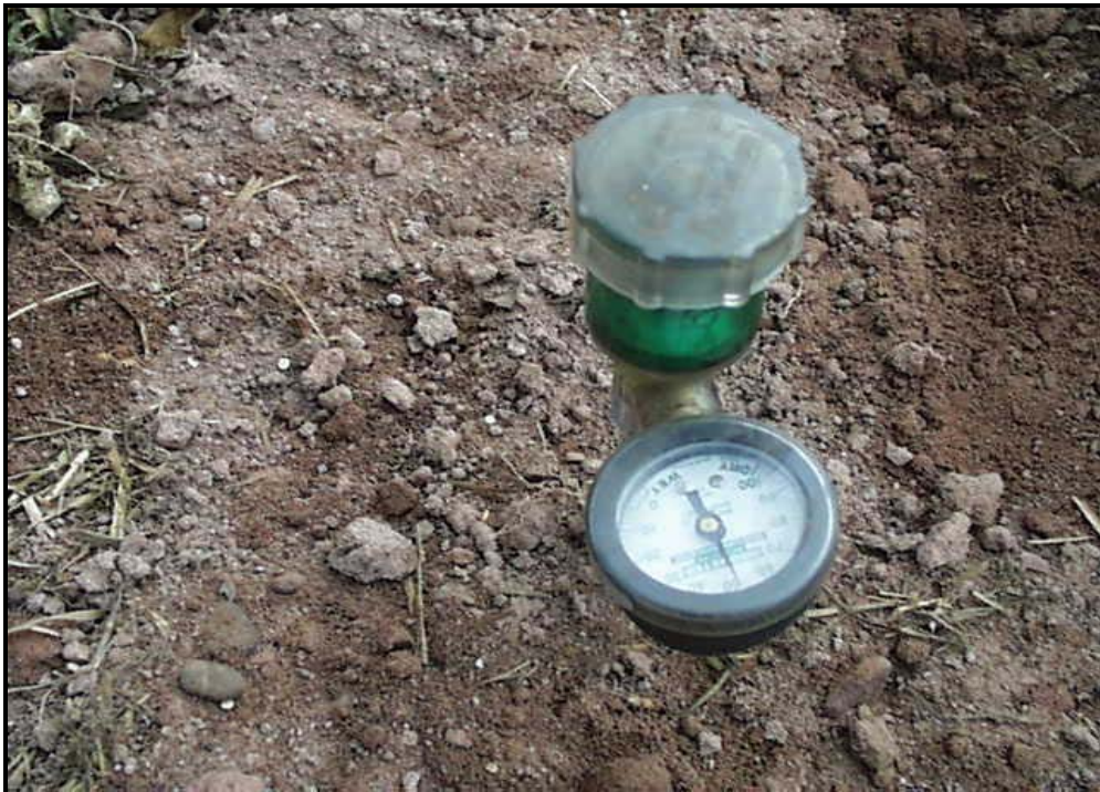
Tensiometers are effective tools to monitor soil moisture levels.
